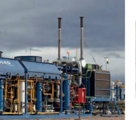
Galileo's 600 horsepower, fourstage Cryobox compressor under construction in Middlesex, New Jersey.
